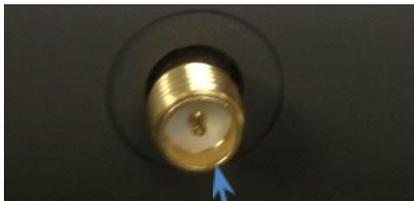
Above, the SMA-M (Reverse Polarity) connector on the back of the D-Link Wireless Access Point. Right of the Wireless Access Point is the SMA-M (RP) connector as well as the Network Port and the Power Connector.
